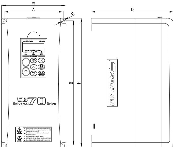
SB70PM18.5~SB70PM375、SB70PM18.5T6~SB70PM315T6挂式单机机型外形图如下：
